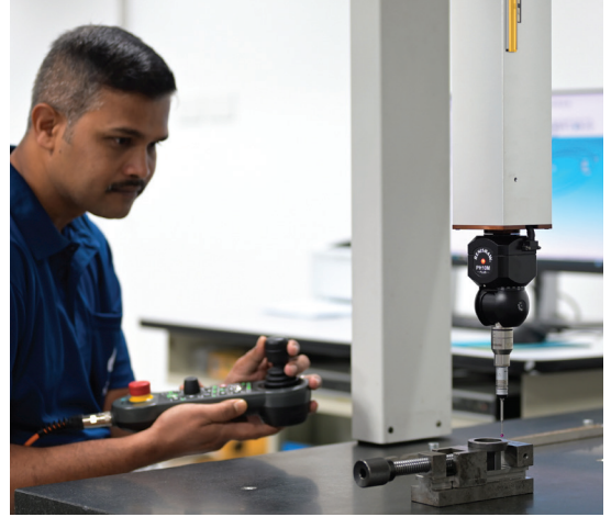
Highly-trained technician carrying out dimensional calibration on complex artifacts.
