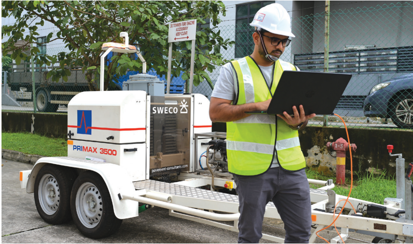
Deployment of heavyweight deflectometer in pavement testing.
