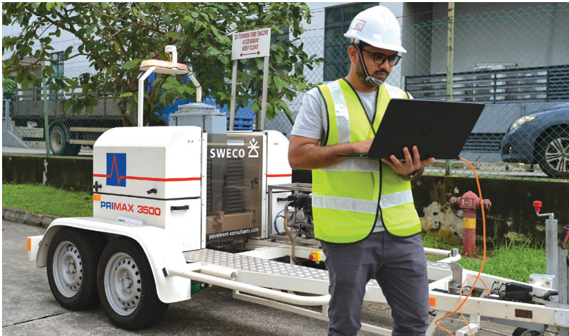
Deployment of heavyweight deflectometer in pavement testing.
