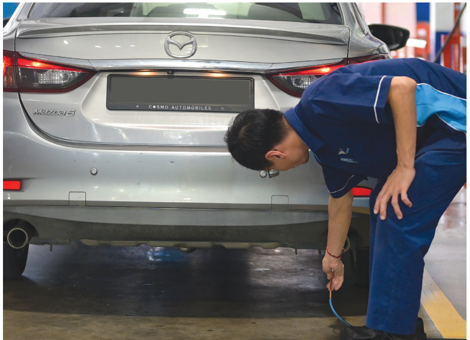
VICOM inspector inserting a probe to measure emissions.
