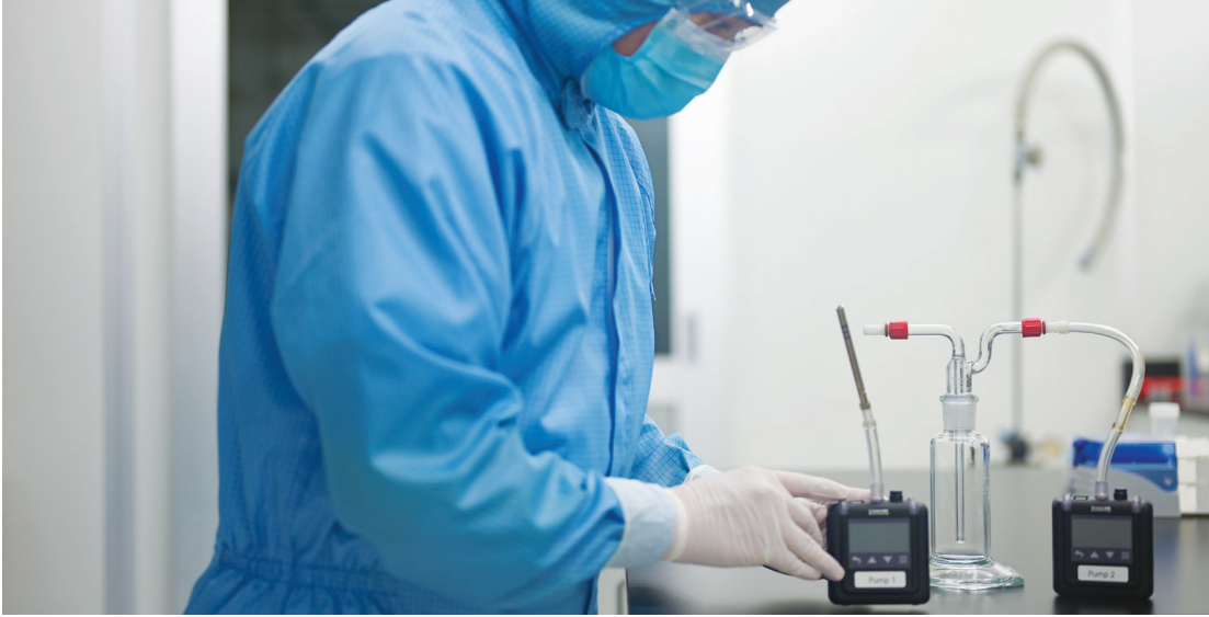
Air sampling with impinger for ion chromatography test.
